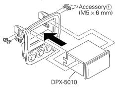
2 Install the center panel with the unit in your car.
